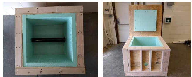
(a) Insulated wooden box used for IRT testing
